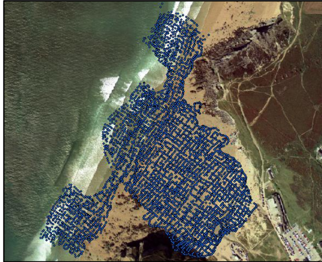
Figure 3.3– Aerial image of PTN, with survey points collected using the RTK GPS mounted on the ATV. Survey date and aerial image are not concurrent, and the two ‘gaps’ in the coverage at the seaward extent of the survey are caused by the presence of two large rip channels present during the survey.
