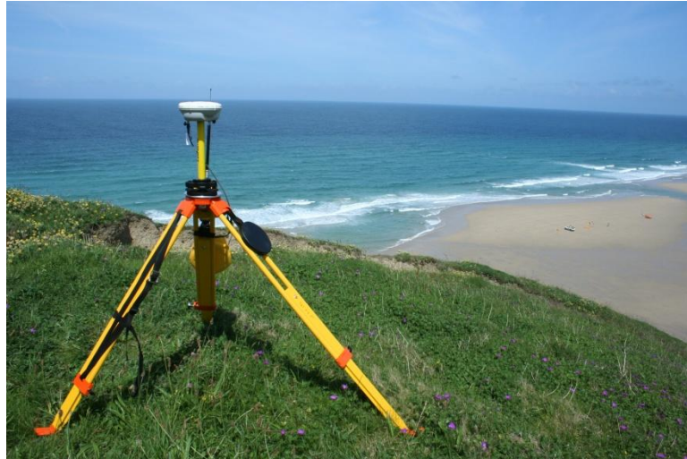
Figure 3.2– RTK GPS base-station sited over a control point at PTN.
