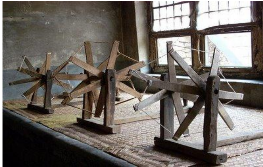
Figure 2.12 The old spinning wheel used to twist fibres together to form yarn [69]
