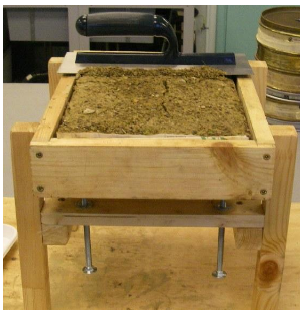
Figure 4.3: Depth increment sampler
