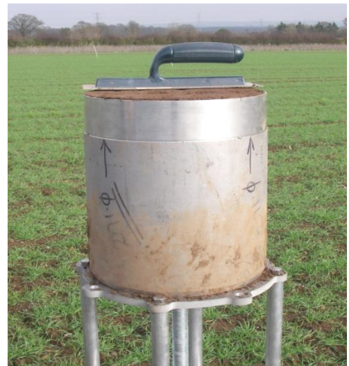
Figure 5.4a: Increment sampler frame showing the base plate and screw which enables the core to be raised at 2 mm increments
