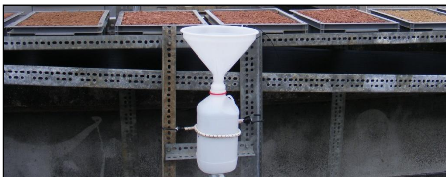
Figure 4.2: Soil trays and rainfall sampler in place on the flat roof
