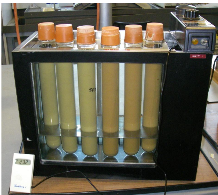
Figure 4.1: Settling columns for determination of clay fractions
