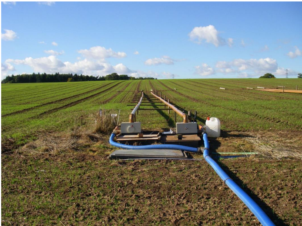
Figure 5.2: Experimental plots and sediment traps used by ADAS UK Ltd (site 2)
