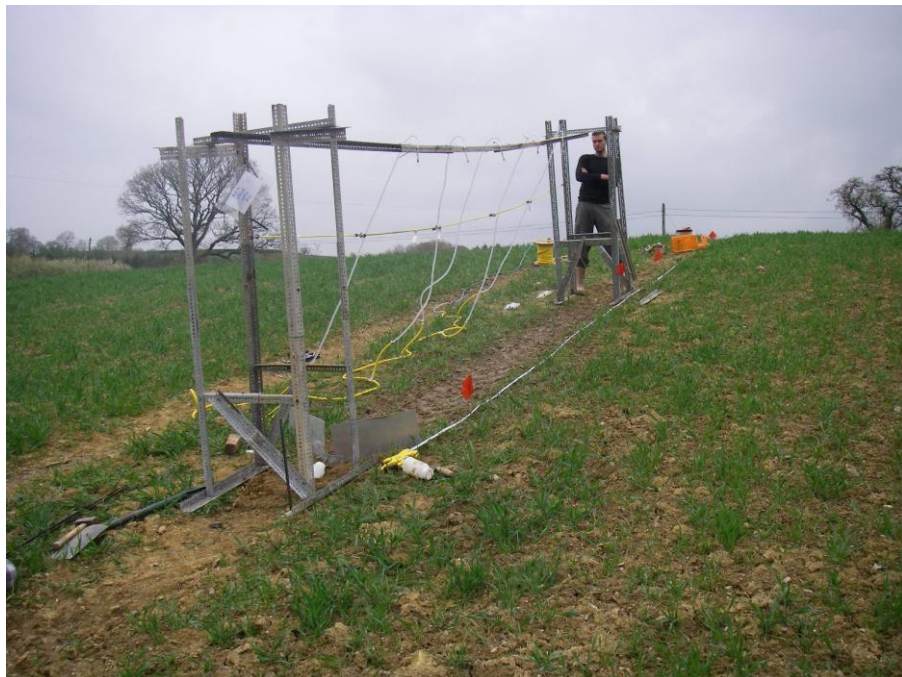
Figure 5.5a: Rainfall simulator erected on the lower 5 m plot
