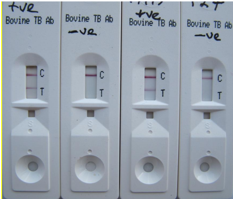
Figure 10 : Four lateral-flow kits showing anti-bovine tuberculosis antibodies test results of four cattle
