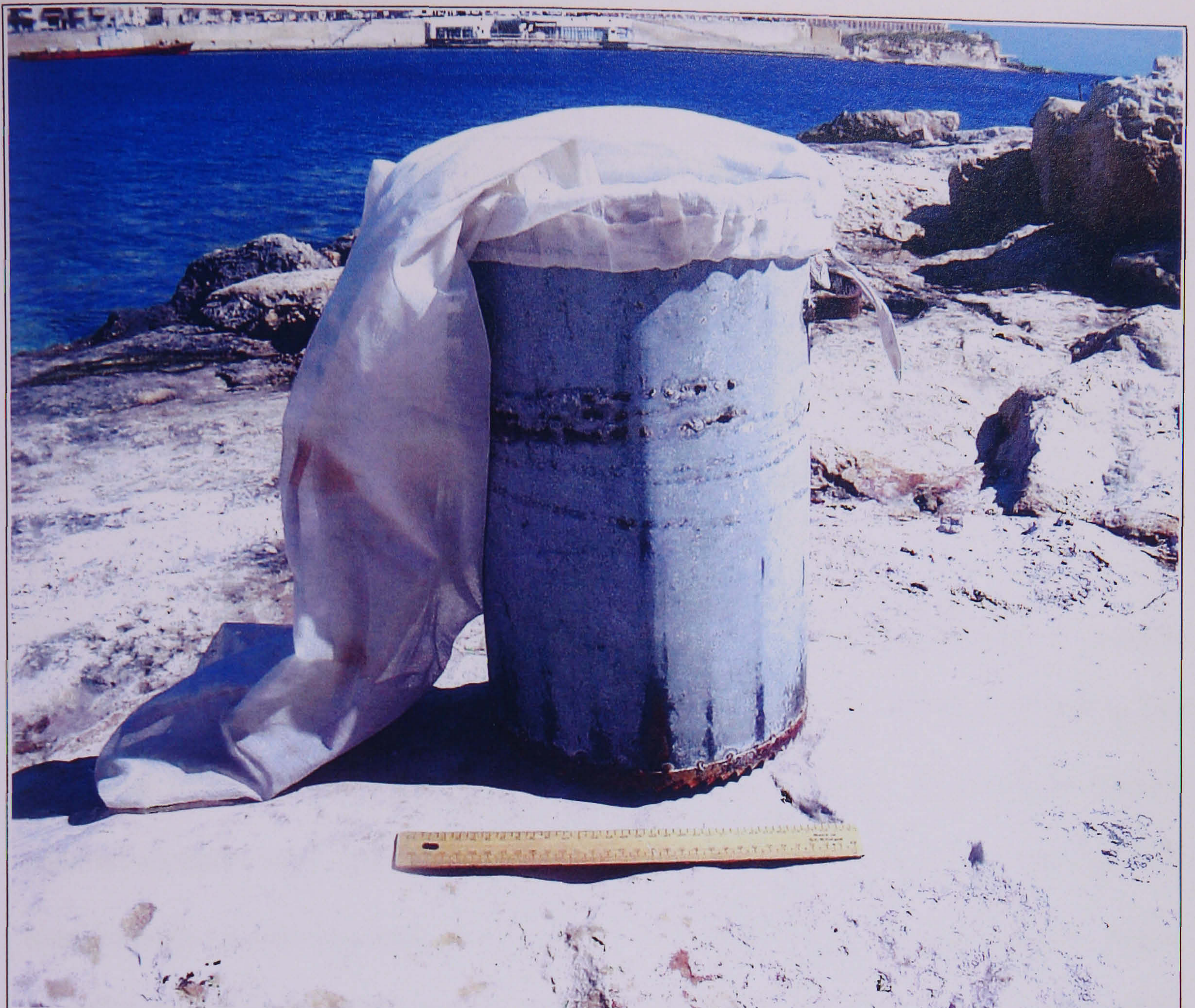
Figure 10. The 25 cm diameter corer with the 0.5 mm mesh collecting bag attached to the mouth. The ruler visible in the photograph is 30 cm long.
