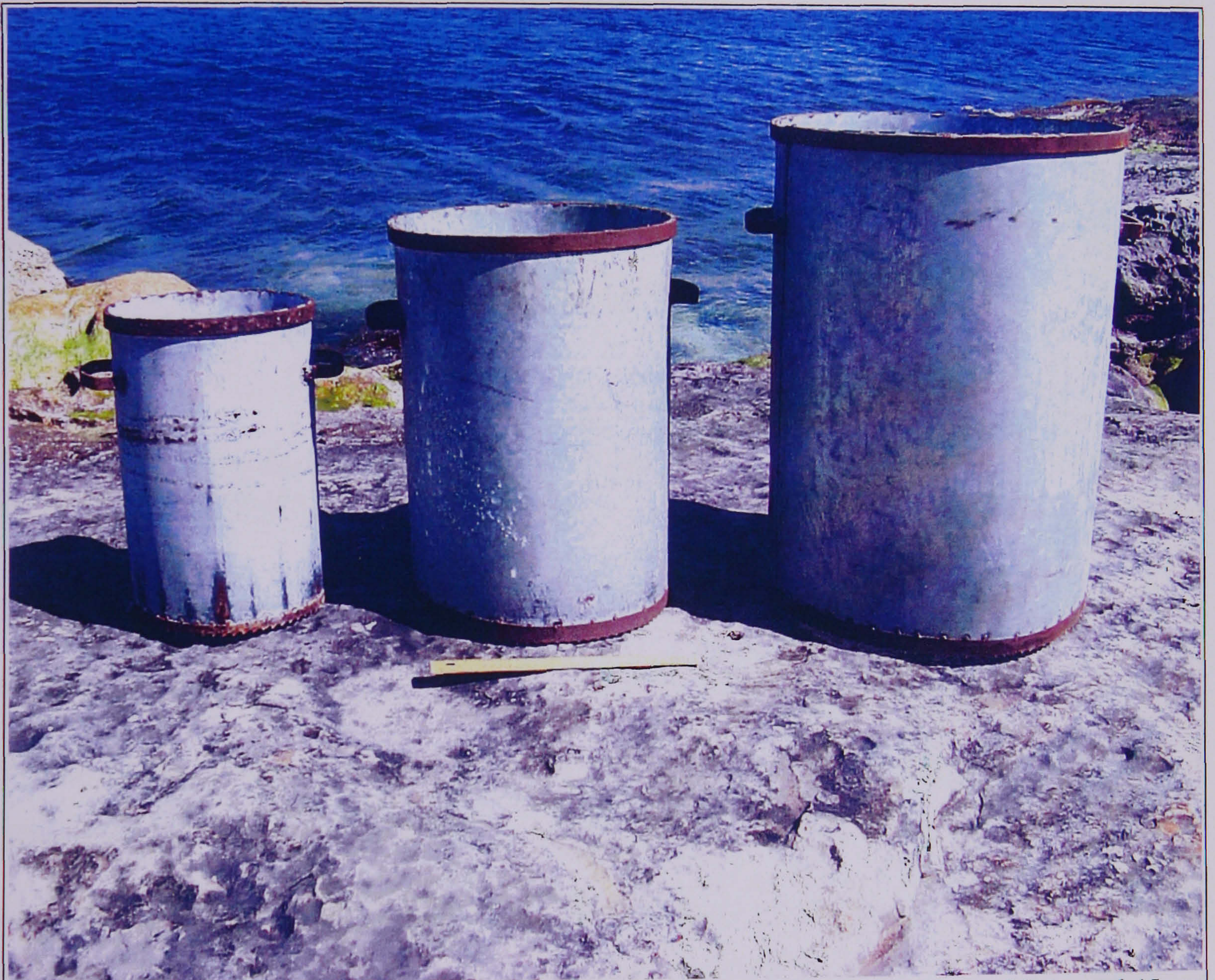
Figure 9. The three cylindrical corers used in the pilot survey; left to right: 25 cm, 35 cm and 45 cm diameter. The ruler visible in the photograph is 30 cm long.
