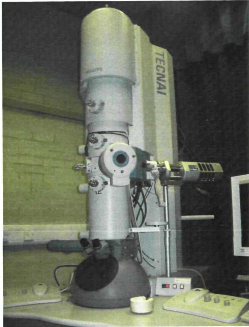
Plate 7.6 Phillips Technai F20 used for TEM analysis.
