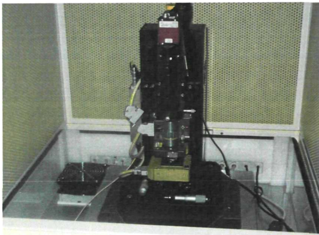
Plate 7.8 XE-100 microscope used for AFM analysis
