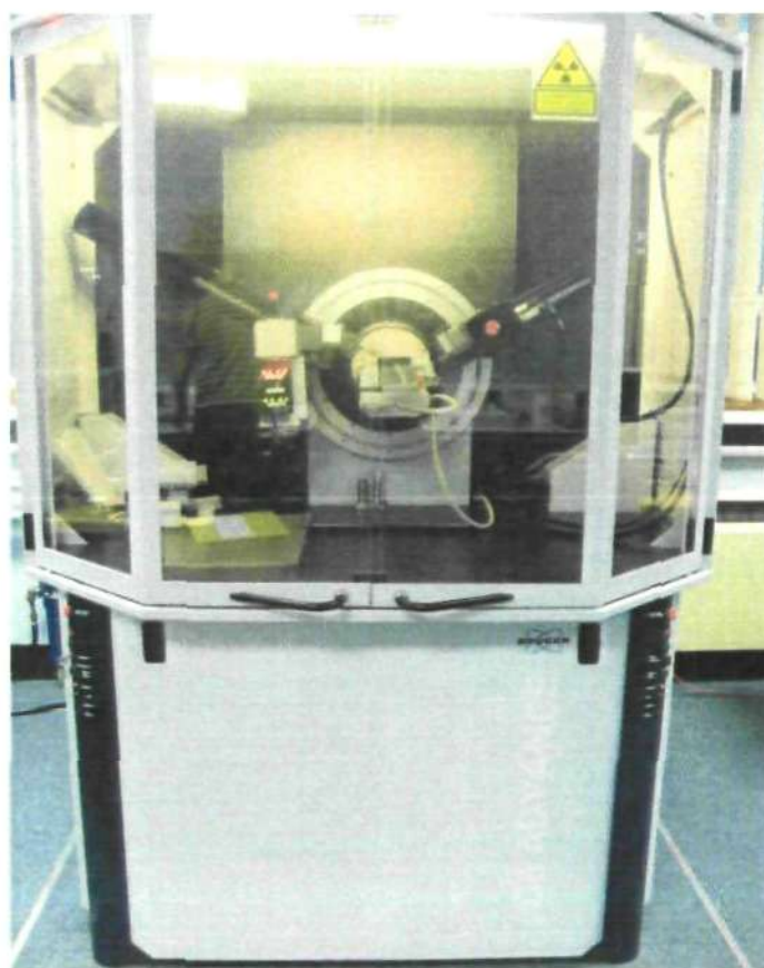
Plate 7.9 Bruker AX D8 used for XRD analysis.
