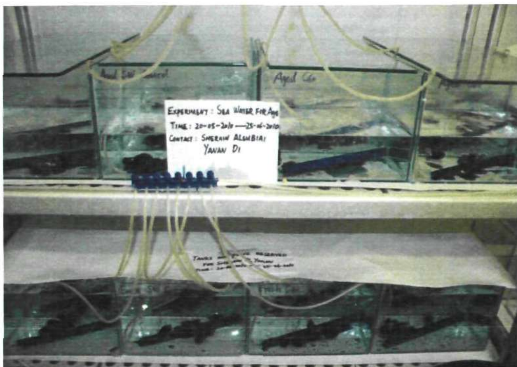
Plate 7.3 Experimental setup for a short-term (3 d) exposure of Mytilus edulis to FSW, ASW, FC 60 and AC 60 in individual 5 L aerated tanks.
