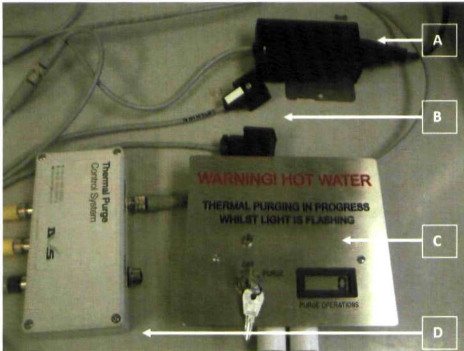
Figure 4.1 Thermal purging unit used during trial, consisting of (A) power supply, (B) solenoid plugs which are simultaneously attached to the solenoids at the top and bottom of each system, (C) key switch unit with digital purge counter, and (D) thermal purge control system.
