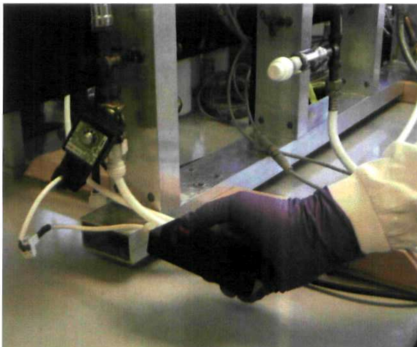
Figure 2.5 Manual flushing of test rig system one using key switch.
