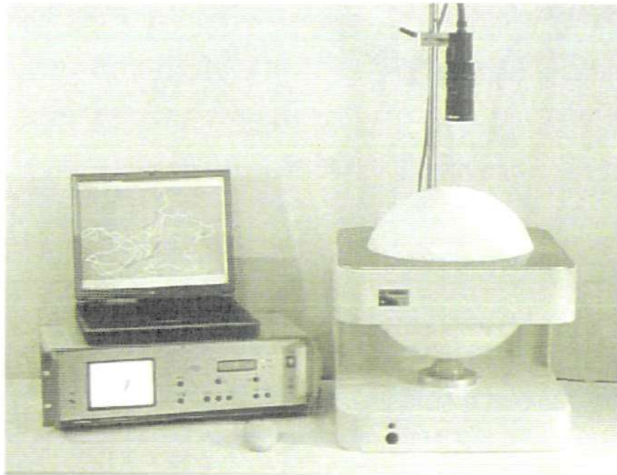
Figure 5.1. Syntech LC-300 locomotion compensator with control unit and portable PC (Syntech, 2004)
