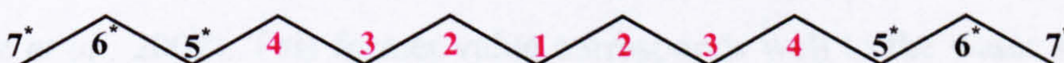
Figure 4.16. Diagram indicating the internal (red) and external (*) isomers of a C 13 alkylbenzene.
