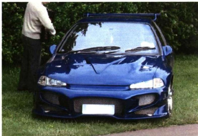
Figure 4: A standard saloon car modified to appear more aggressive. Note the lowered suspension, wide bodywork and meshed ventages
