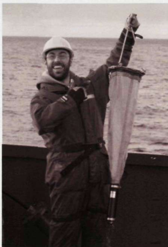
Figure 6.3-3. One of the plankton nets used for collecting vertical water column samples from the chlorophyll a maximum region to the surface; Diameter; 30 cm, length; 50 cm, mesh; 20 \mu\text{m} .
