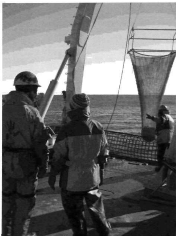
Figure 6.4-1. Agassiz sled used for collecting macrofaunal (> 1 cm) specimens from sea floor sediments; Length 250 cm; width 40 cm; mesh size 1 cm.
