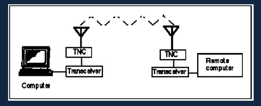
From its first steps in Montreal, Canada, in 1978, to its current AX25 protocol implementation established in 1982 by the Amateur Radio Relay League of America, packet radio provides the means through which computer data may be transmitted, error free, on the radio frequency spectrum. It represents one of the fastest growing areas in amateur radio today.
