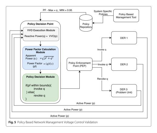
be implemented using PBNM. The PDP would validate the Power Factor (PF) against the relevant policy supplied by the policy database and, if the bounds are violated, the system would trigger the *policy obligation* within the policy to request an updated VVC from the 3-OPF tool. One more check would then take place to verify the PF against the policy to determine if the issue has been resolved by this operation. If not, the updated VVC would
