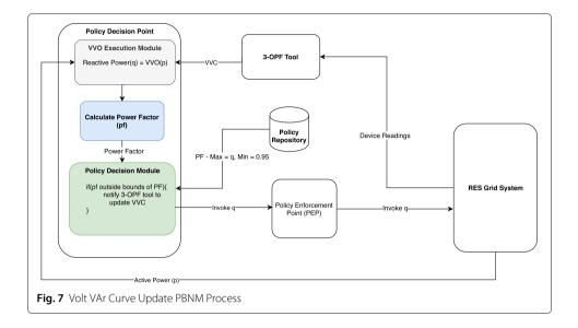
be used to calculate the reactive power set point to be sent to the inverter to stabilise the Power Factor. One of the advantages of the combined AVM-PBNM approach is that the current manual process could be automated, so voltage stability could potentially be restored much more quickly, and not in 5 minutes as is the case in this test.
