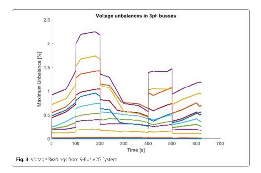
network state is unacceptable so the PDP triggers a policy that instructs the AVM component to create an updated VVC. The new VVC is deployed at the RES at 14:58, thereby restoring voltage stability. Meanwhile the bounds applied to the generation of the VVC can be maintained to ensure that the Power Factor does not exceed the Leading Power Factor ensuring acceptable voltage quality.
