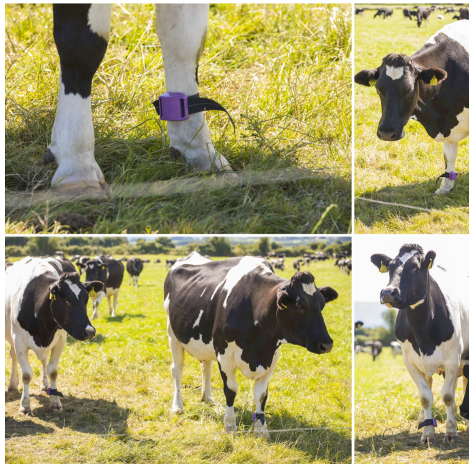
Fig. 1: Pedometer attached as a part of the experiment to the front leg of the cows
