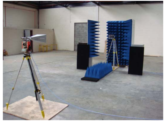
Figure4. Large hall test configuration, without wooden frame
