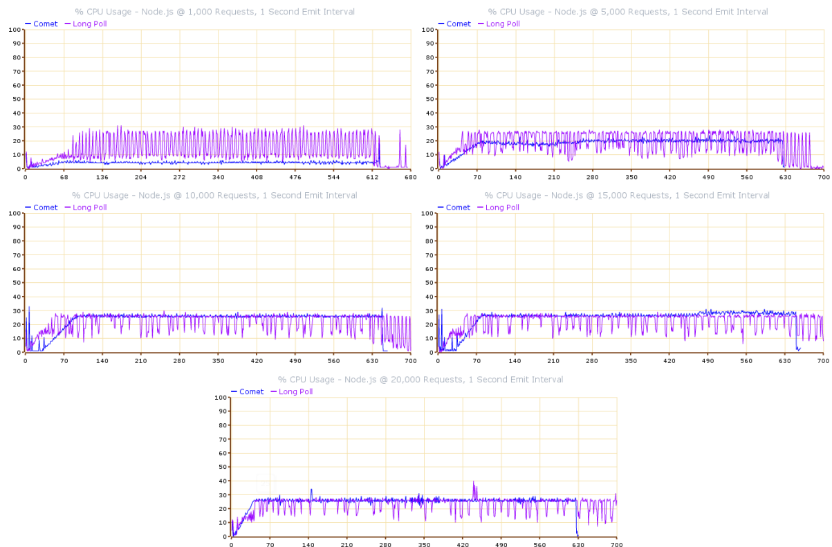
Figure 17: Node.js – Comet vs Long Poll – 1 Second Emit Interval – CPU Usage.
