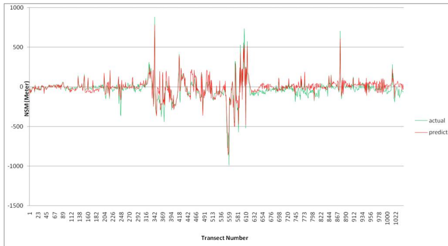
Fig. 5 — Actual and predicted shoreline movement in 2015 from the baseline along Andhra coast
