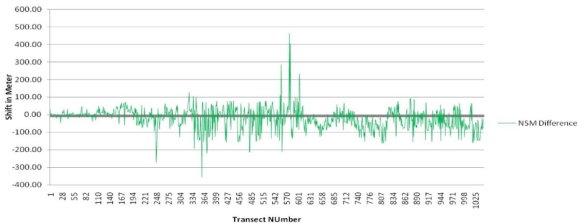
Fig. 6 — Positional shift in between actual and estimated shoreline of 2015
