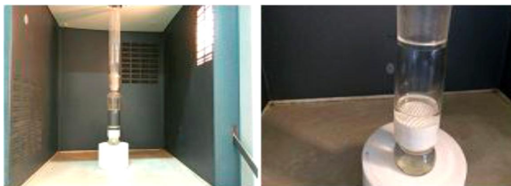
Specially designed glass reactor for microwave assisted honeycomb catalytic reactions.
