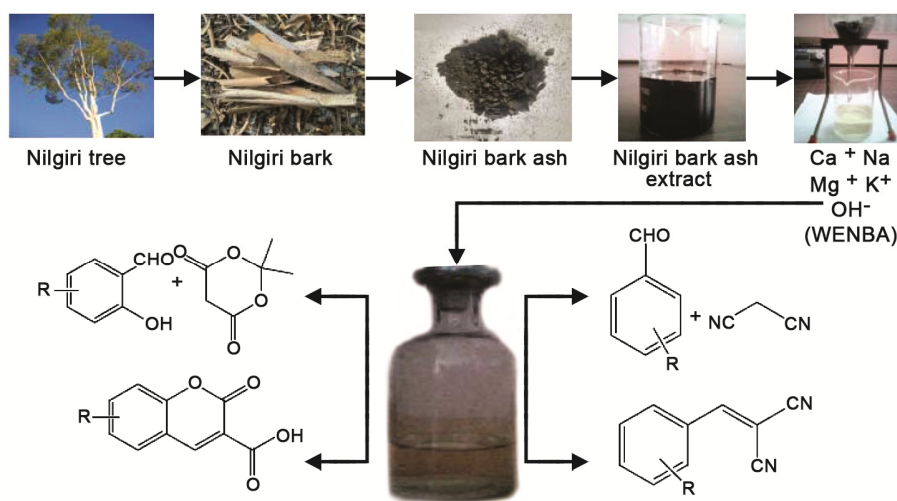
Scheme III — Preparation of WENBA and its catalyzed synthesis of coumarin-3-carboxylic acid and arylidenemalononitrile derivatives
