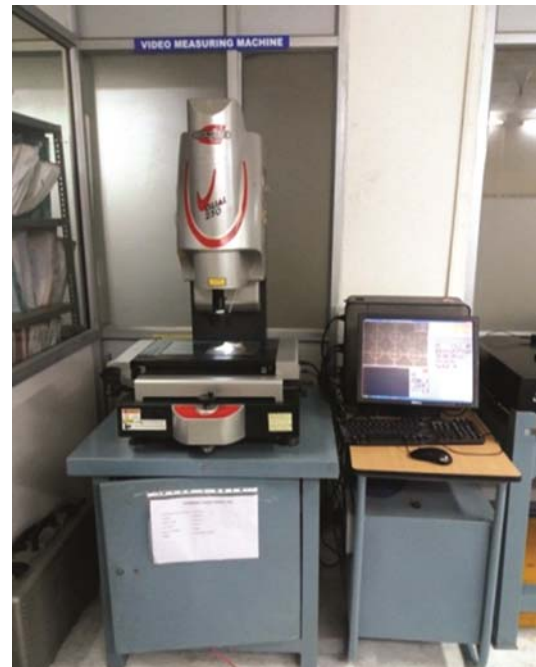
Fig. 2 — Video measuring machine used for formability measurement.
