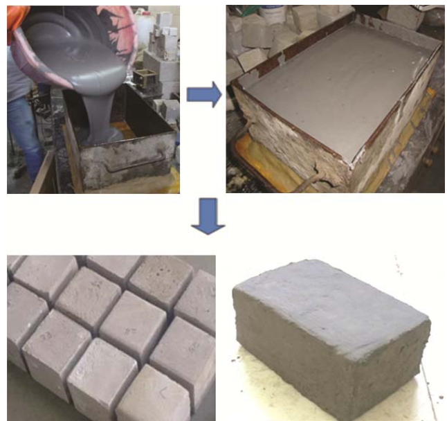
Fig. 13 — Production of the foamed geopolymer concrete blocks.
