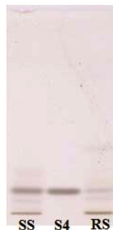
Fig. 6 — HPTLC profiles of the methanol extracts of roots of rainy season (RS) and summer season (SS) and standard shatavarin-IV (S4) visualised at white light after derivatisation
