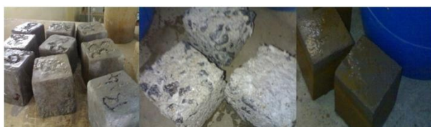
Fig 10 — Specimens before immersion and after immersion in the sulphuric acid and hydrochloric acid
