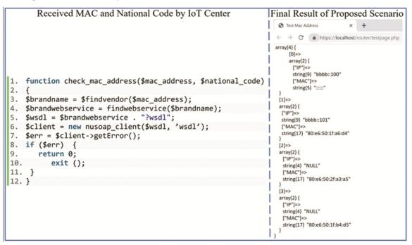
Fig. 2 - Received MAC and National Code by IoT Center, and Final Result of Proposed Scenario
