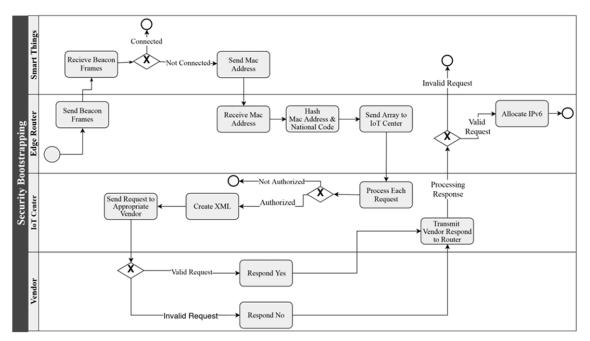
Fig. 1 — BPMN Model of the Proposed Method
