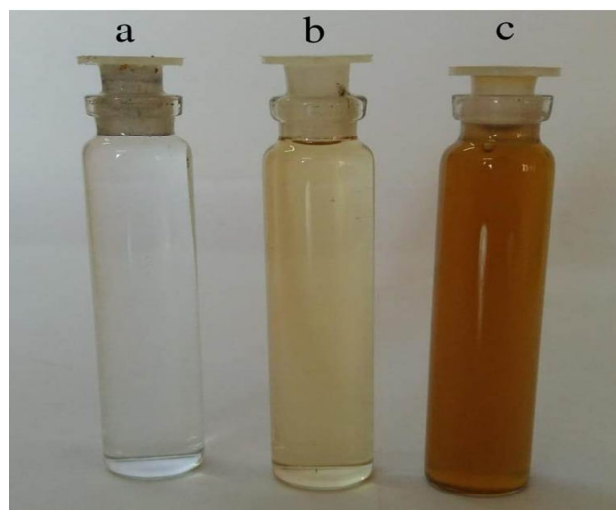
Fig. 2 — (a) Magnesium nitrate solution, (b) aqueous extract of Rhizophora lamarckii , and (c) magnesium oxide nanoparticles synthesized using R. lamarckii
