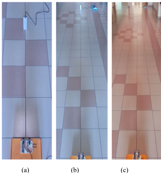
Fig. 6 — Experimental set-up of received signal strength (a) 1 m, (b) 5 m, and (c) 10 m
