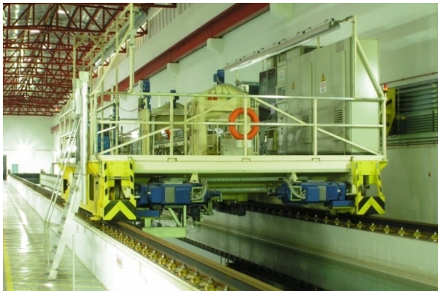
Fig. 5 — Towing tank Carriage UTM
