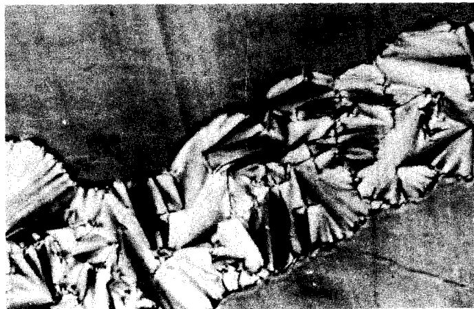
Plate 2—Induced smectic-A phase, fan-shaped textures, (131.2°C), crossed polarisers ( \times 150 )
