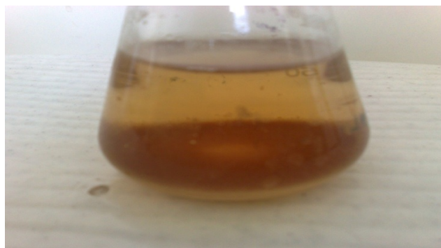
Fig. 8 — Chromium in the treated tannery effluent is settled at the bottom by chemical precipitation
