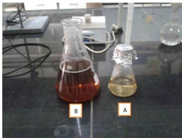
Fig. 1 — The aqueous extract of N.zanardinii (A) before; and (B) color change after synthesis of Ag-NPs
