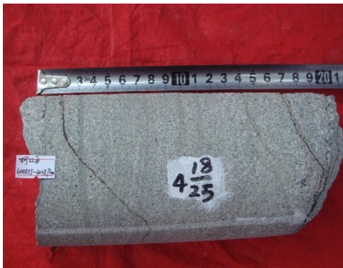
a. Low angle shearing cracks, Ke22, 4008.55m~4008.74m
