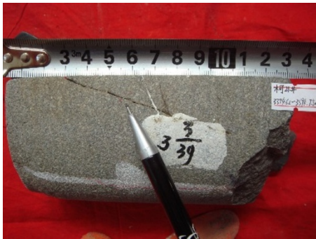
b. High angle shearing cracks, Ke21, 3394.62m~3394.75m
