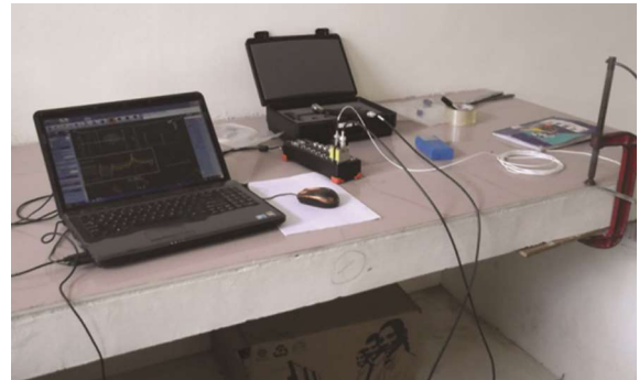
Fig. 1 — Setup for modal analysis
