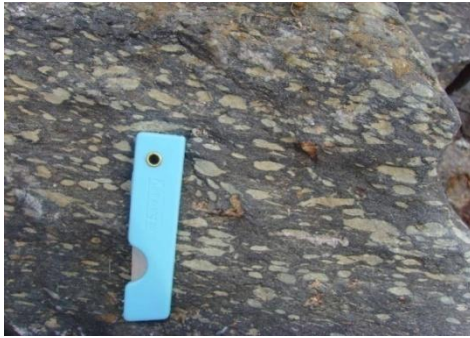
Fig. 2-Metabasalt of Zhaertai Group (with amygdaloidal structure)
