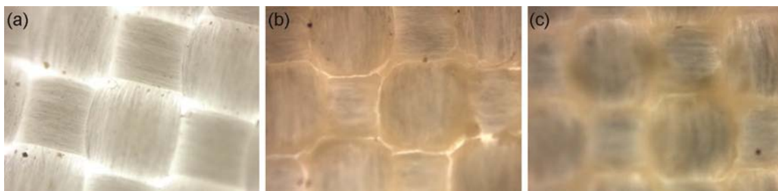
Fig. 3 — Microscopic images of samples after drop test [(a) non-treated Dyneema, (b) 34% STF treated Dyneema, and (c) 38% STF treated Dyneema]
