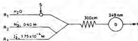
Fig. 1—Schematic diagram of the flow injection system
