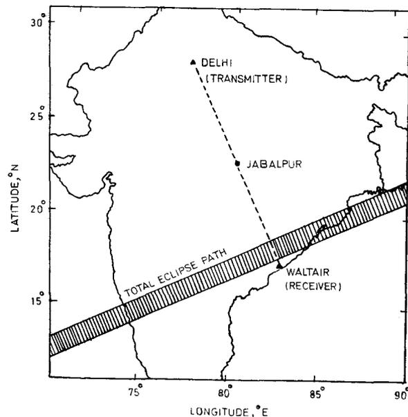
Fig. 1—Map showing the locations of the transmitter, receiver and the approximate reflection point and a rough sketch of the totality path of the total solar eclipse of 16 Feb. 1980
