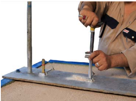
Figure 10: Piles installed in the model.
