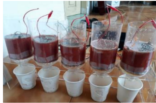
Gambar 3. Wadah Proses Electroosmosis Dewatering
