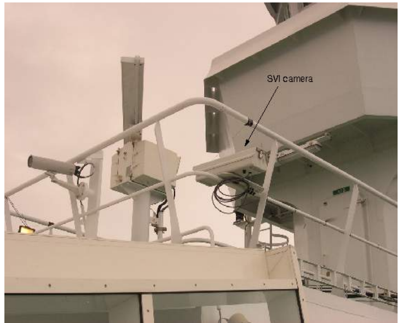
Figure 12. The SVI camera clamped to the railing on the lower radar platform.
