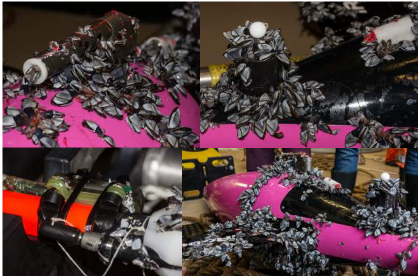
Figure 9. Photo's displaying the biofouling on all glider sensors directly after retrieval.
