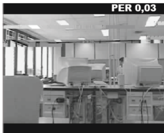
Figure 9. Image A with PER = 3% and image B with PER=10% with restart marker
