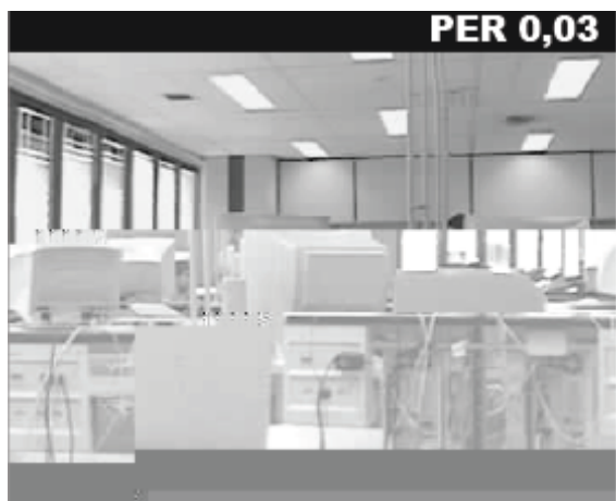
Figure 10. Image A with PER = 3% and image B with PER=10% without restart marker
