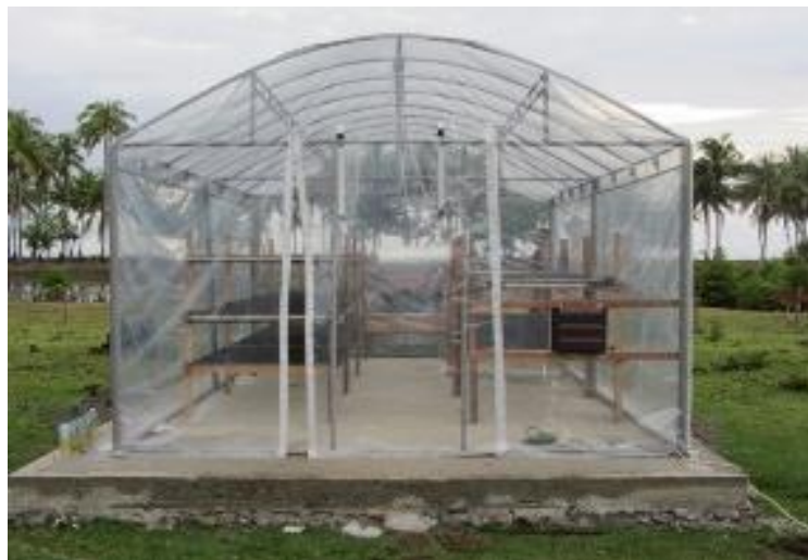
Fig1. Greenhouse solar dryer chamber
