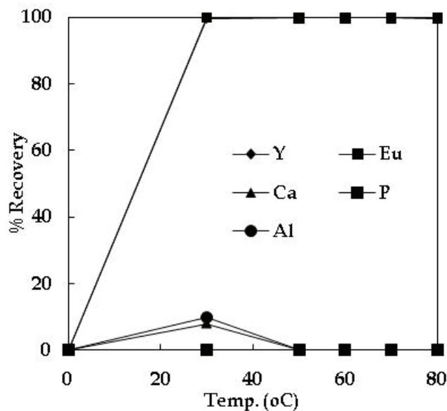
Figure 3. Effect of temperature on precipitation of rare earths.
