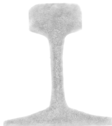
Fig. 6 : Sulphur print of processed Rails from stirred bloom
