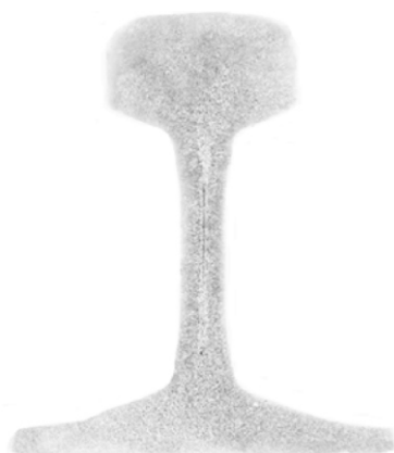
Fig. 5 : Macro of processed Rail from unstirred bloom
