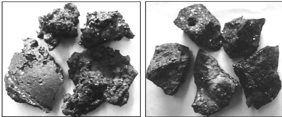
Fig. 4 (a & b) : Photographs of post de-sulphurised slag samples a) Base period - metallic & heavier, and b) Trial period - brittle & light
