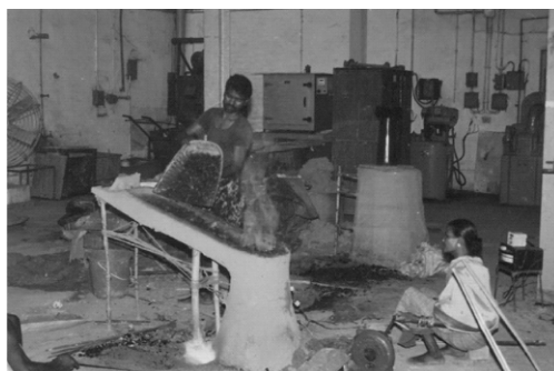
Fig. 1: A glimpse of proto-type furnace (Bastar model) in operation
