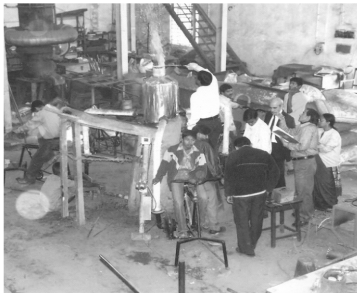
Fig. 3 : Scaled-up furnace (Bastar model) with heat recovery system in operation.
