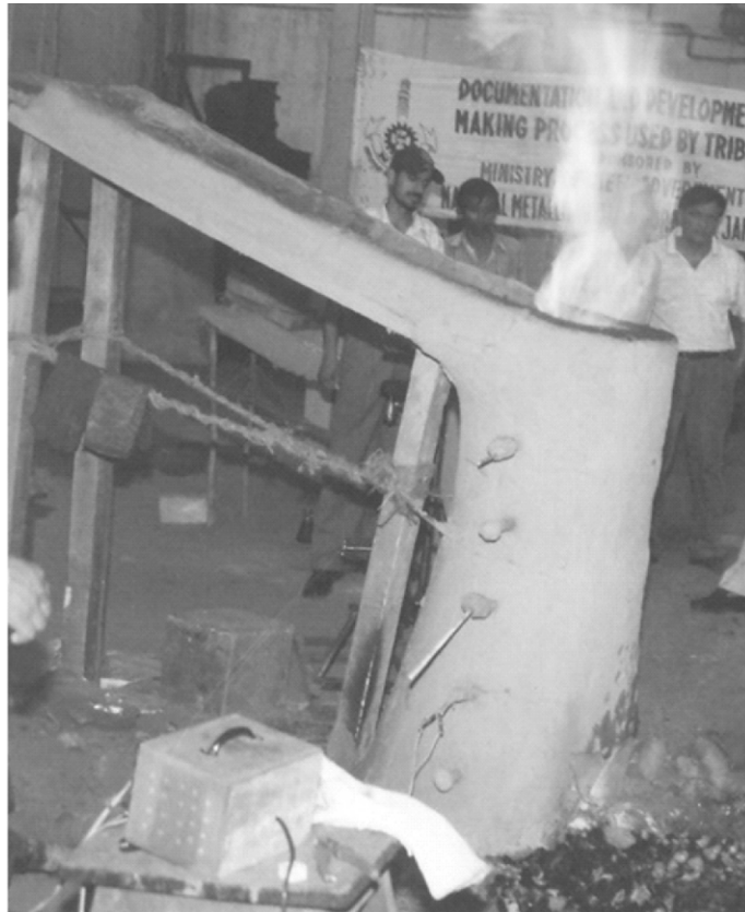
Fig. 2 : Scaled-up furnace (Bastar model) without heat recovery system in operation.
