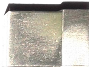
Fig. 7: Diffusion bonded specimen W/Ti/SS processed at 1000°C, 5MPa and 15 min
