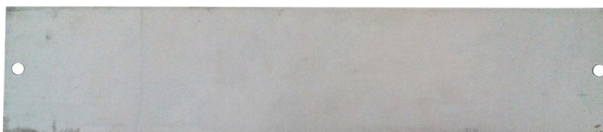
Fig. 3 : Specimens for strip annealing simulations in Gleeble
