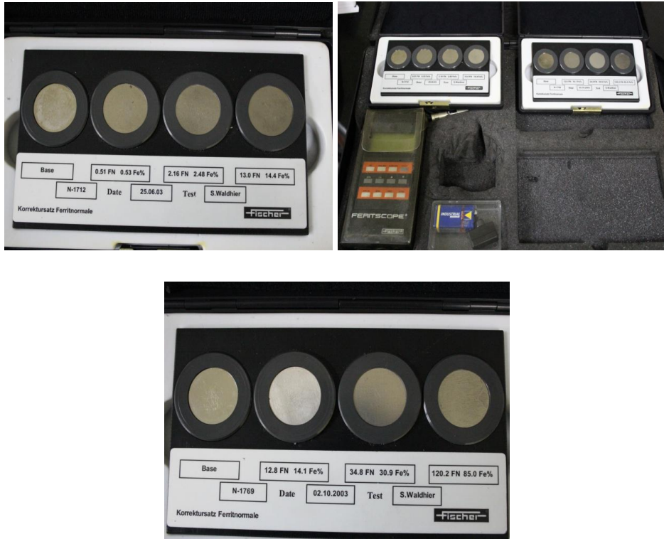
Fig. 5: Ferritscope arrangement with reference samples of different ferrite content for calibration
