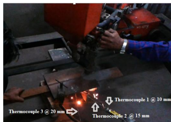
Fig. 2: Performing test welding by SAW Process
