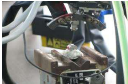
Fig. 3: Performing Residual Stress Analysis of AISI 1035 steel raw material
