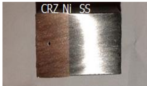
Fig. 4: Diffusion bonded specimen SS/Ni/CRZ processed at 1000C, 5MPa, 15 min
