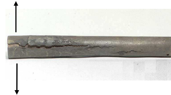
Fig. 12. Jacket around cooling pipe. Circumferential hoop stresses are responsible for cracking along the pipe length
