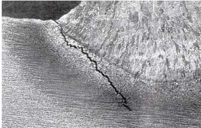
Fig. 24. Cold cracking near a weld
