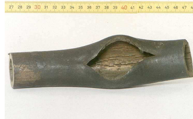
Fig.26. H Attack in a condenser pipe http://sirius.mtm.kuleuven.be/Research/corr-oscope/hcindex2/tutor21.htm
