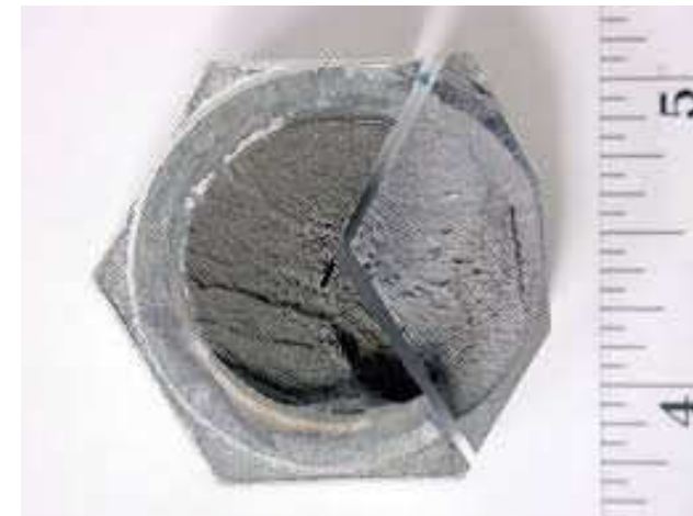
Fig. 21. HE can result in extremely brittle cracking as shown here for a screw which has failed within a nut
