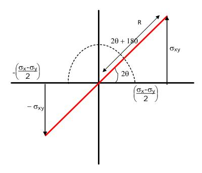
axis is  $(\sigma_{xy})$  then the plane of consideration will make an angle  $tan2\theta$ . This is illustrated in the figure below.
