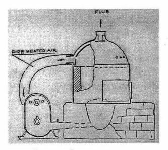
Figure 3. Schematic sketch of the fuel efficient furnace
