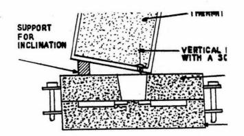
Figure 1. Schematic Figure of obtaining metal block from thermit melting
