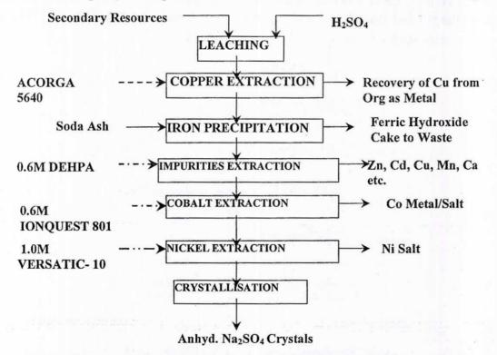
Fig-4 : SX process for the recovery of metals/salts from secondary resources
