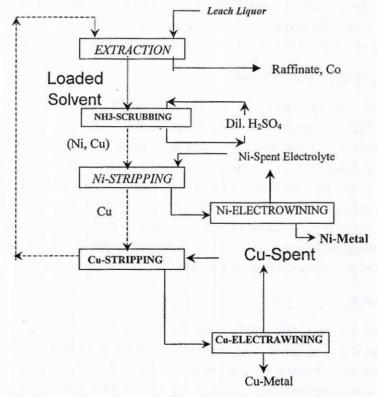
Fig-5 : Separation of metals from leach liquor by solvent extractionelectrowinning (SX-EW)
