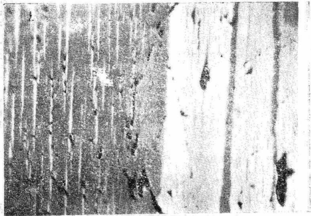
FIG. 11—A grain showing both exsolved haematite (white) in ilmenite (dark grey) and ilmenite in haematite. Beach sands of Orissa Coast.
